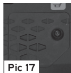
16. Engine Oil Filler Cap Access Panel
