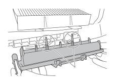
If the filter is difficult to remove, hook the filter with the tab on the filter cover to make it easier to remove.
