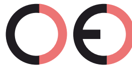
False CE Mark (too far)
