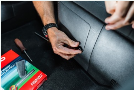
STEP 3 Remove locking clip that was held in by phillips screw.
