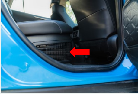
STEP 1 Location of battery air filter is on drivers side, underneath rear passenger seat.
