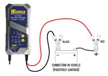
If Positively Earthed – FIRST Connect the Black (-) Crocodile clip or ring terminal lead to the (-) battery terminal and then connect the Red (+) Crocodile clip or ring terminal lead to the vehicle's chassis. DO NOT connect the Red (+) lead to the carburettor or fuel lines.
