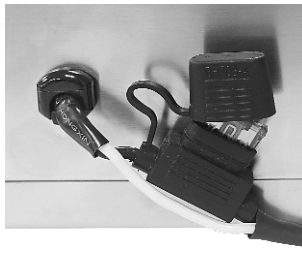
15A Replaceable inline fuse protection
