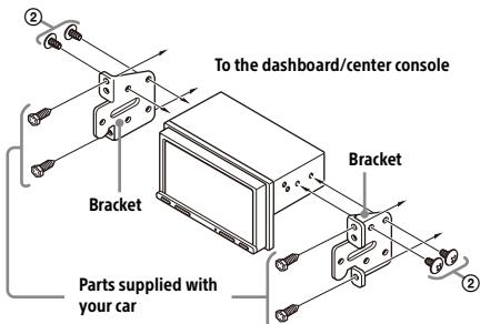
When mounting this unit to the preinstalled brackets of your car, use the mounting screws ② in the appropriate screw holes based on your car:
