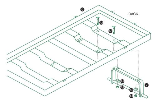
Then attach the top part of the Rear Axle Support (Part 7) to the base (Part 6) using bolt parts A1, A2 & A3 as pictured to the left.
