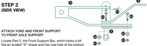
Locate Part 5, the Front Support Bar, which looks a bit like an angled "S" shape and has one hole at the bottom and two holes at the top.
