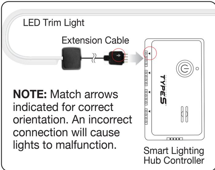
**NOTE:** Match arrows indicated for correct orientation. An incorrect connection will cause lights to malfunction.
