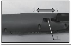
To prevent the switch lever from accidentally pulled, the lock lever is provided.
