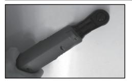
Hold the tool firmly and place the socket over the bolt/nut. Turn the tool on and fasten. When the bolt/ nut reaches the seating position, the tool stops automatically.
