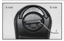
This tool has a reversing lever to change the direction of rotation. Turn the reversing lever to the A side for clockwise rotation or to the B side for counterclockwise rotation. Make sure that the reversing lever is fully turned with a click.
