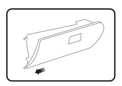
1. The cabin air filter housing is located in the passenger footwell at the end of the centre console. The main wiring harness tray has to be dropped to gain access.
