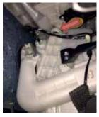
3. Grab the old cabin air filter and pull it out gently from the housing to avoid any accumulated debris from spreading around.
