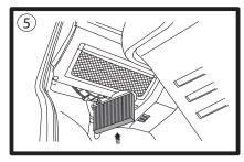
Push new Ryco RCA112M filter into housing.
