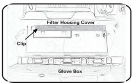
3. Replace old cabin filter with RYCO RCA242M and ensure the air flow arrow is pointing to the floor. Refit filter housing cover and glove box. Dispose of used filter correctly.
