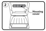
2: Remove housing cover by unclipping ends and pull out.
