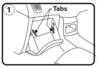
1: Partly open glove box and remove the 2 tabs, let glove box hang down out of way.
