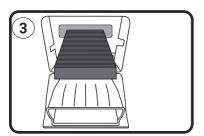
3:Remove used filter and replace with a new Ryco filter. Note direction of flow arrow printed on filter.
