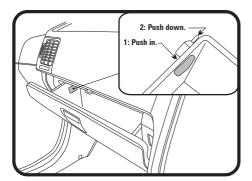
Open glove box and remove retaining pins on either side of glove box, then fully open glove box.
