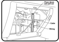
2: Remove cable and wiring from filter cover plate, push down and pull out to remove cover plate.
