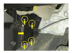
The cabin air filter location is on the drivers side footwell at the far end of the centre console. To access the filter undo the 4 screws shown in the picture with a Phillips screw driver and remove the housing lid.
