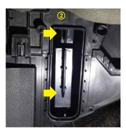
Once the cabin air filter housing lid is out of the way, the filter will be accessible. Pull the first filter out and then reach for the second one. Pay attention on how the filters sit in and replicate this with the new ones, making sure they are placed in the right air flow direction. Lastly refit the housing lid.
