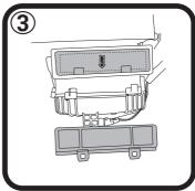
Unclip filter cover and remove, pull used filter out of housing and replace with new Ryco filter.
