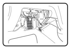
2: Remove 5 screws & 2 hex head bolts from 4: Dispose of used filter correctly. around glove box frame, gently pull glove box out until plug for glove box light is visible and disconnect. Remove glove box to expose cover for cabin filter. Remove cover to gain access to filter by pulling out.
