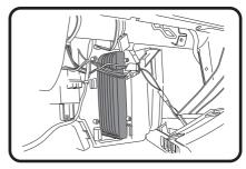
3: Hold wires away from front of housing, Pull used filter out from housing and replace with new Ryco RCA104M filter and re-assemble all previously removed components.
