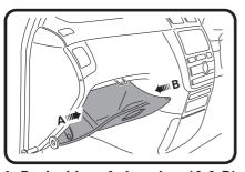
1: Push sides of glove box (A & B) to release catches, roll glove box down, unclip hinges to remove glove box.
