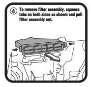
Beamove used filter from tray, fit new filter to tray making sure that flat side is facing down.
