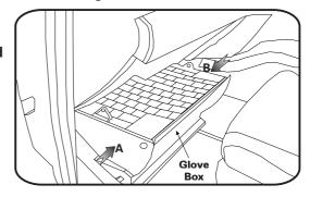
2. The cabin air filter housing is located above glove box. Remove the cover by squeezing the clip located on its right side.
