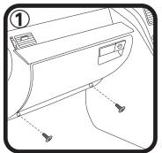
Undo 2 screws at bottom of glove box as shown.
