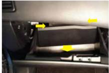
With the strut unclipped, proceed to release the glove box from its securing hinge. Simply apply some pressure to the far upper corners towards the inside of the compartment as indicated in the pic and slowly drop the unit.
