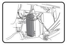
3: Hold wires away from front of housing, Pull used filter out from housing and replace with new Ryco RCA104P filter and re-assemble all previously removed components.
