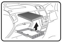
3: Remove used filter from tray. Fit new Ryco filter. Refit all previously removed components.
