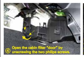
GUD Automotive Pty Ltd 29 Taras Ave Altona North Victoria 3025 Australia. www.rycofilters.com.au Remove the old filters. Insert the new filter with foam on its top and push up into the compartment. Slide and snap the other filter and refit all parts in reverse direction.
