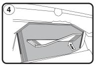
4: Clean debris from inside filter housing, Slide the new filter into housing.
