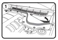
1: Starting at passenger side peel weather strip back to the end of plenum cover ("A")
