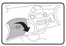
1: Open glovebox, apply pressure to both sides of glovebox to release catches.
