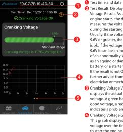
Page 1 Test Result: Displays Cranking Voltage Result. As the engine starts, the device measures the voltage level during the starting process Usually, if the voltage is 9.6V or greater, the system
