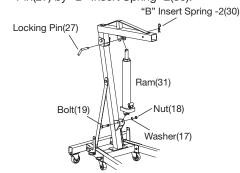
11. Slide the Boom Extension(32) into the Boom and use the Locking Pin(27) and "B" Insert Spring -2(30) to secure at the desired load rating. Use the Bolt(37), Washer(33) and Nut(34) to attach the Hook and Chain(35) to the end of the Boom Extension(32).
