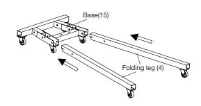
5. Folding Leg (4) in place using the Pins(6). To insert the Pins, lift up on front of Base(15) until holes line up. After all two Pins(6) are inserted, insert "B" Insert Spring-1(8) through small hole at end of each Pin until it snaps into place. Then use two Bolts(12), Flat washers(11), Spring washers(9), Nuts(10), Bolts(19), Flat washers(17), and Nuts(18) to fasten the Fixing plates(13).
