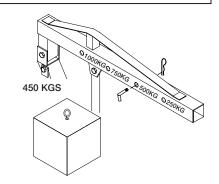
2. Adjust the Boom Extension so the hole on Boom Extension aligns with the chosen hole on the Boom. Secure into place by inserting the Locking Pin through aligned hole and securing in place with the R-Clip.
