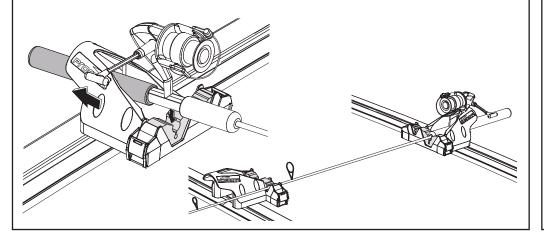
To secure rods, push the Zip Straps into the Buckles on either side of the Rod Holders.
