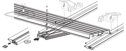
Position the Rod Holder Bodies on each crossbar with the strap/foam ends pointing towards each other. Secure the Rod Holder Bodies to the Slot Nuts in the crossbars using the M6 Button Head Capscrews 12mm and M6 Spring Washers via the rear holes as shown. Tighten to 4Nm with 4mm Allen Key Screwdriver provided or a suitable Torgue Wrench.
