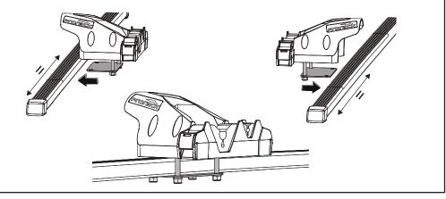
To secure rods, push the Zip Straps into the Buckles on either side of the Rod Holders.
