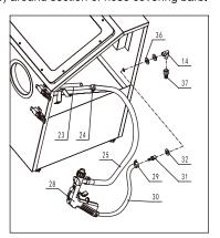
**Step 4:** Connecting siphon hose(25) onto sand suction tube(23) tightened by siphon hose clamp(24).
