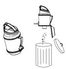
Press the automatic release button to empty the dust into dust container.
