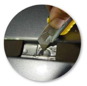
• To reveal the screw thread in the mounting points, remove the sealant covering them with a sharp tool.
