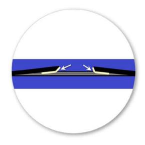
Remove one side of adhesive tape backing. Apply to underside of rubber insert as shown. Remove second backing, then apply downward pressure onto vehicle.
