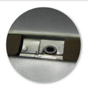
If crossbars are removed, please install the rubber plugs into the ditch moulding.
