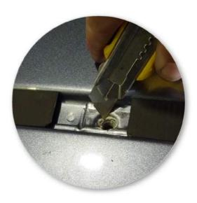
• Remove sealant as shown.
