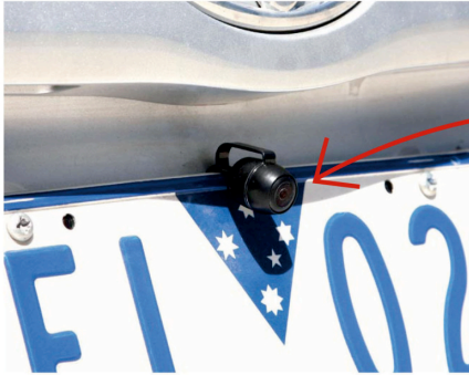
Installation example of stealth camera.
