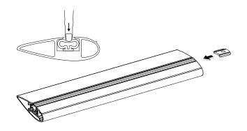
Using two shorter M6 x 16mm capscrews, two M6 spring washers and two M6 washers, assemble awning bracket or other accessory mount as shown.
