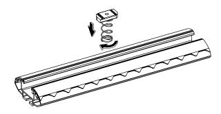
Using two longer M6 x 20mm capscrews, two M6 spring washers and two M6 washers, assemble awning bracket or other accessory mount as shown.
