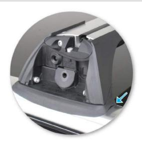
Ensure back edge of foot sits flush with the back edge of vehicle roof rail.
