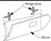
1: Open glove box, remove hinge pins by levering out as shown, remove glove box.
