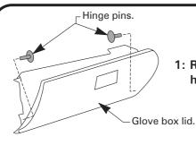
1: Remove glove box lid by levering hinge pins out as shown.
