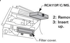
2: Remove filter cover, remove used filter.
