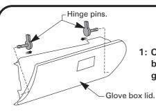
1: Open glove box, remove hinge pins by levering out as shown, remove glove box.
