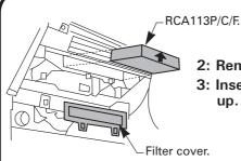
2: Remove filter cover, remove used filter.
