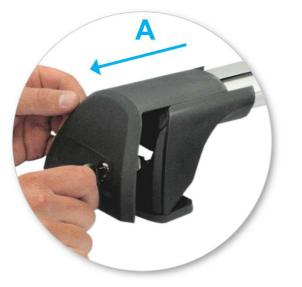
• For type A, remove cover with keys.
