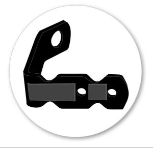
Cut grey protective strip to size. Apply as shown.
