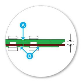
Loosen both screws on the clamp so there is a gap between part A and part B.
