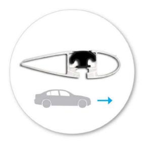
Ensure the roof rack face towards the front of vehicle.
