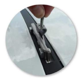
Select four internal clamps and fit them to the inside of the installed clamps on the vehicle.
