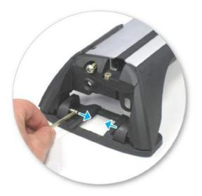
Remove both pins from each leg. Use tapered end of spanner located inside left hand cover to assist.
