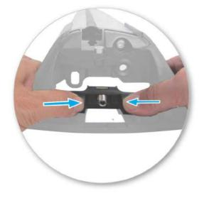
Remove plastic clamp block by gripping bar leg with fingers and push firmly with thumbs until clamp block drops out behind leg.
