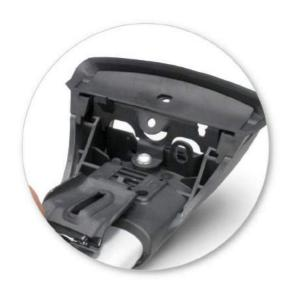
Remove crossbar off vehicle and turn upside down. Select metal clamp and fit small tongue into position 1 marked on the leg.
