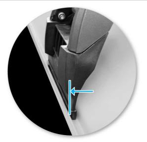
Loosely position crossbar ensuring the guttermount blade is hard against the inside of the vehicle gutter.
