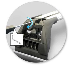
Tighten adjusting screw to 2 Nm (1.5 ft lb) hand tight.
