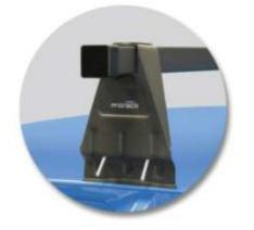
Insert two M6x35 carriage bolts through each leg. Place assembled bar on roof of the vehicle and position legs in gutter ensuring that the crossbar is positioned evenly across the vehicle, i.e. similar length of crossbar protruding from each leg.
