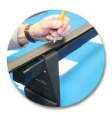
Place rubber infill on the open crossbar channel with one end pushed against a leg and mark with a pen to cut at the other.
