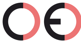
False CE Mark (too far)
