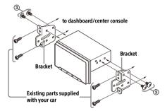
When mounting this unit to the preinstalled brackets of your car, use the mounting screws ③ in the appropriate screw holes based on your car: T for TOYOTA and N for NISSAN.
